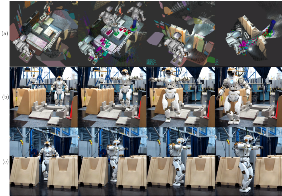
Fig. 3. A collage of the main locomotion tasks. The top row of subfigures (a) show the operator's view with the superimposed planar regions and the planned footstep paths for both the uneven terrain task and the narrow gap task. The footstep planner is able to snap desired footsteps onto the detected planar regions, avoid unsafe footholds such as potholes, and plan paths through a narrow passageway. The middle and bottom rows (b) and (c) subfigures show a snapshot sequence of uneven terrain traversal and narrow gap crossing respectively.
